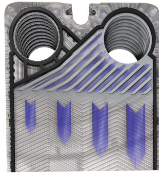
Conventional Design Distribution Low velocity at the far corner reduces plate performance.
